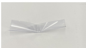
Etirement Vs élongation. Apparition de D-cônes
